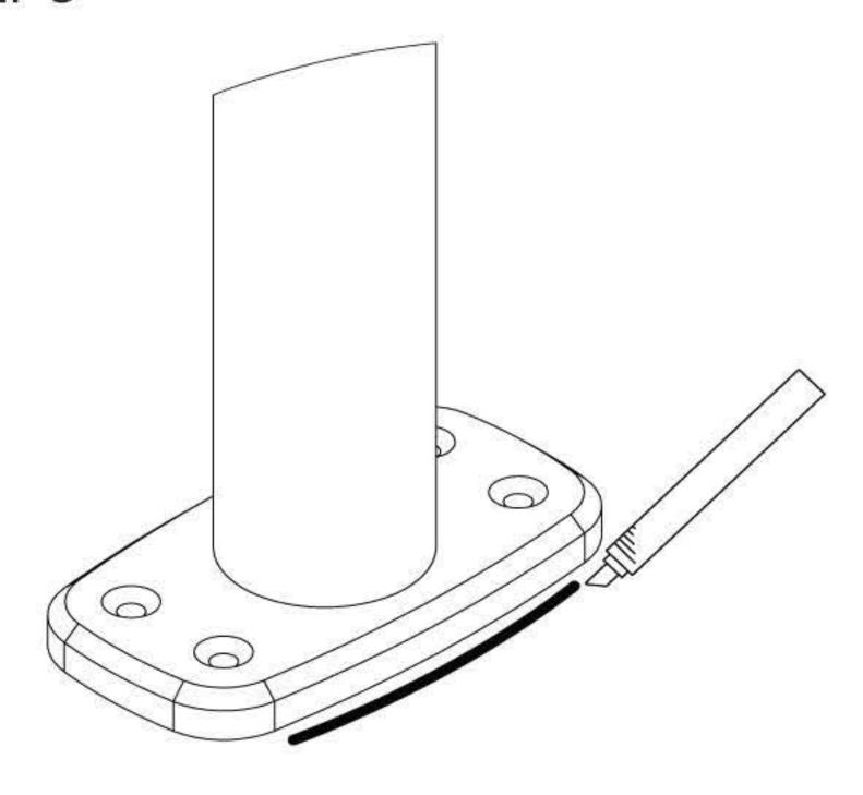
USE A MARKER TO MARK OUT WHERE THE FEET ARE POSITIONED.
