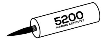
Apply a generous amount of marine grade sealant on the deck matching the contact patch of the mounting feet.
